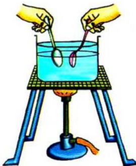
Comparison of Thermal Conductivity of Steel and Plastic
