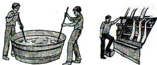
Scouring in Tanks
